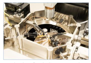
Sample Probe Configured with 2 RF + 2 COAX Probes
